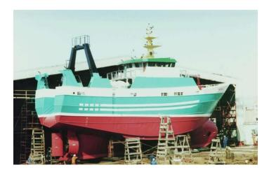
**Type** Stern Trawler of single chine hull form with transom stern,
